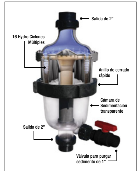
Partes del Pre-filtro Multi Cyclone
